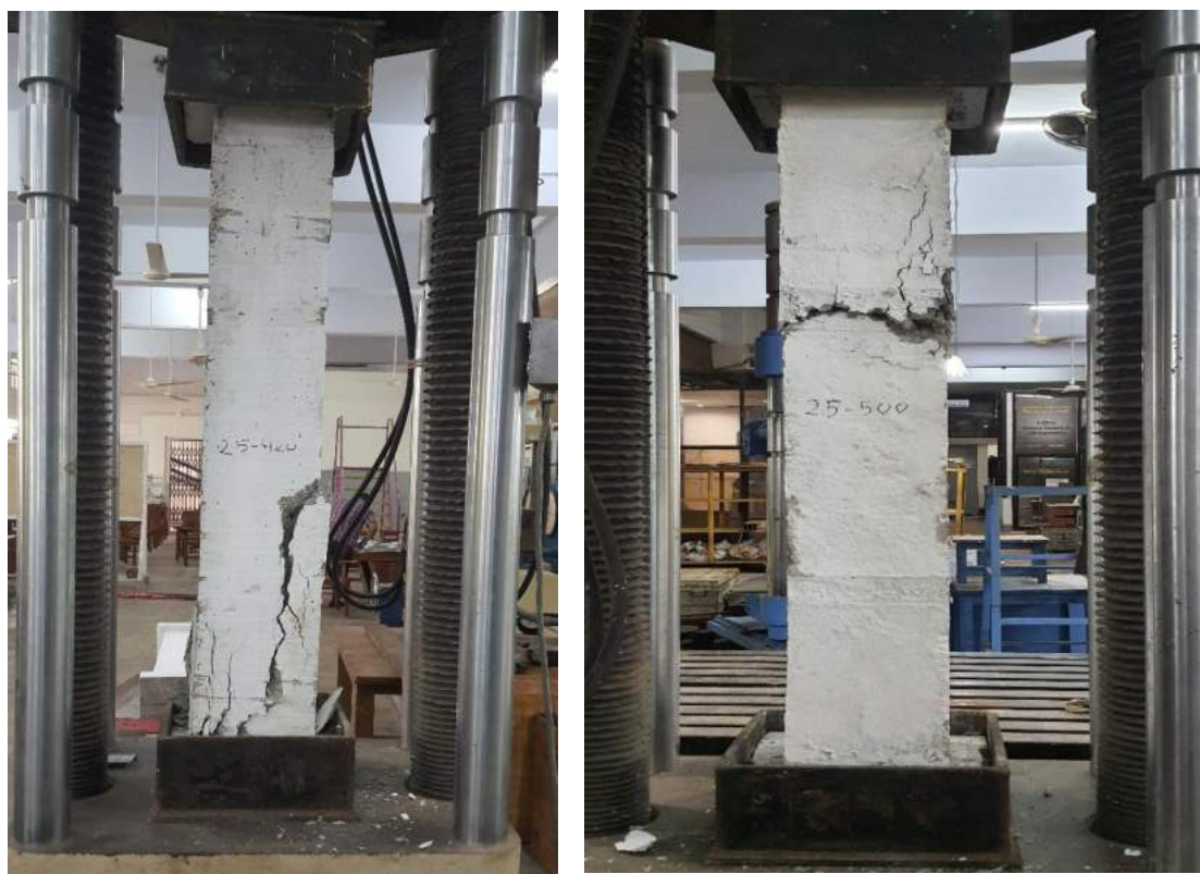
Figure 3.34: Failure patterns of column reinforced with (a) B420DWR (b) B500CWR
