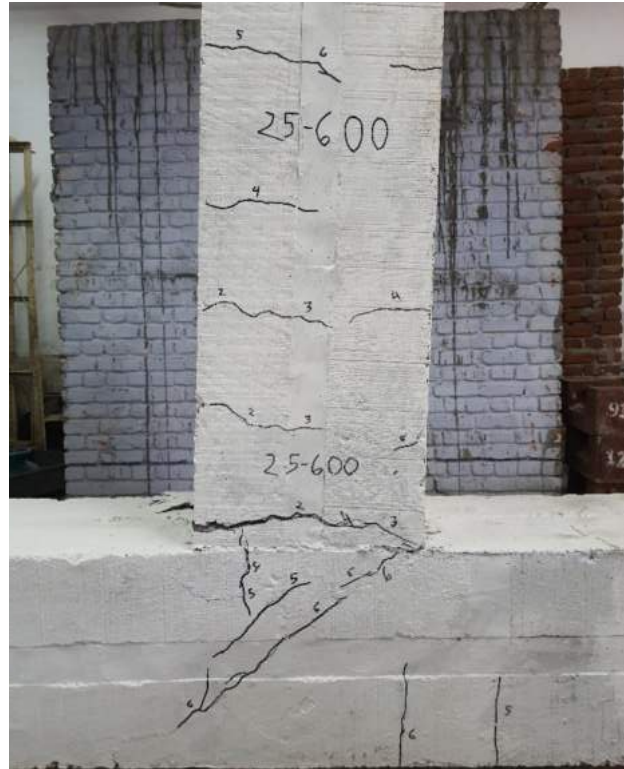
Figure 3.48: Cracking characteristics of joint reinforced with B600C-R
