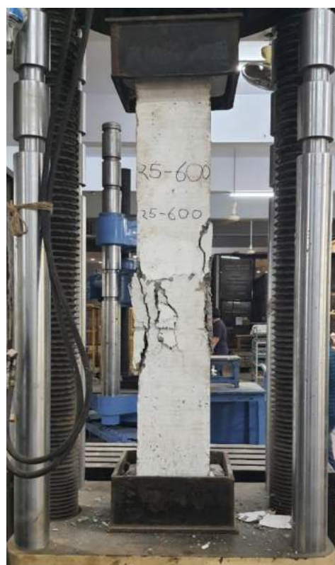
Figure 3.35: Failure patterns of column reinforced with B600C-R
