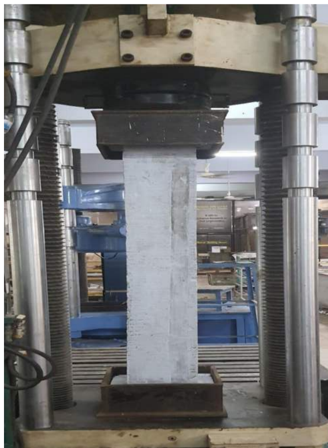
Figure 3.31: Test set up of column for concentric axial load in laboratory
