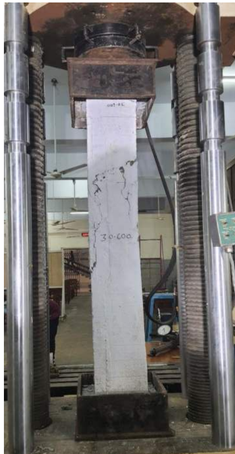
Figure 3.37: Failure patterns of column reinforced with B600C-R
