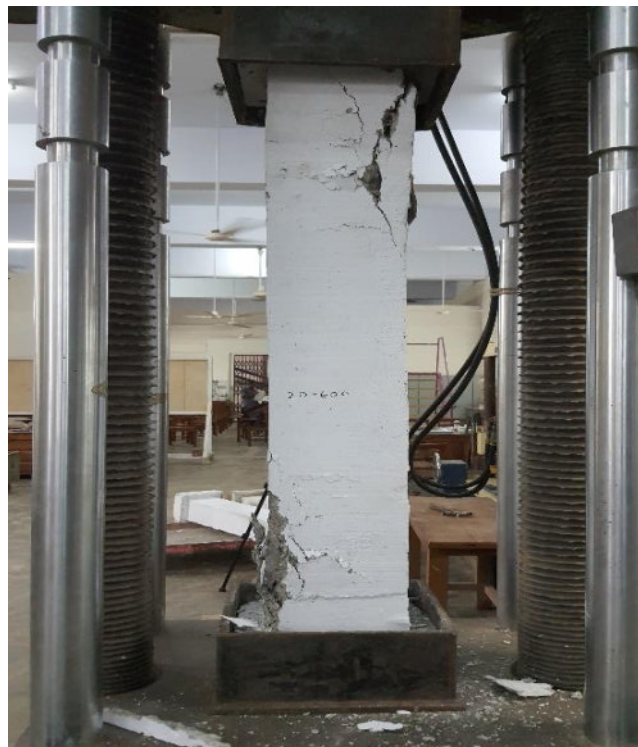
Figure 3.33: Failure patterns of column reinforced with B600C-R
