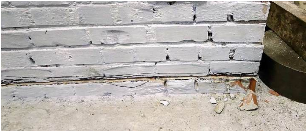
Figure 4.6- Cracks at final state of HURM4 (Rocking).
