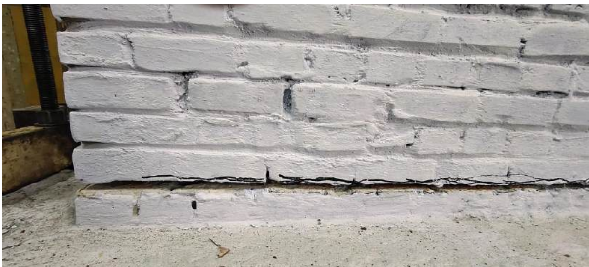
Figure 4.2- Cracks at final state of SURM4 (Sliding).
