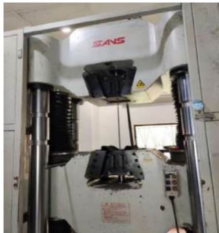
Figure A.1- Testing of rebar.
