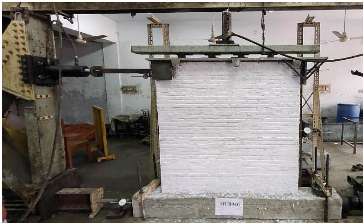
Figure 3.36- Full experimental setup of masonry wall
