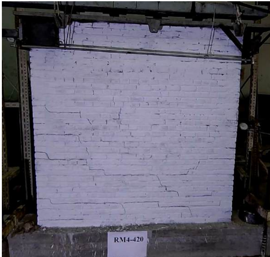
Figure 4.9- RM4-420 after the completion of cycle 7.
