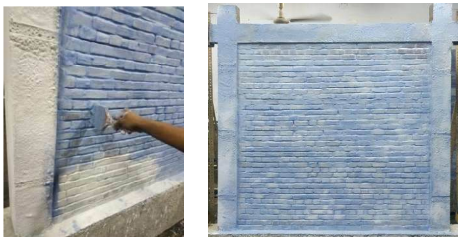
Figure 3.29- Infilled Frame after whitewash.
