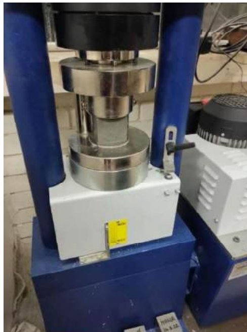
Figure D.1- Prepared mortar cubes mortar testing.
