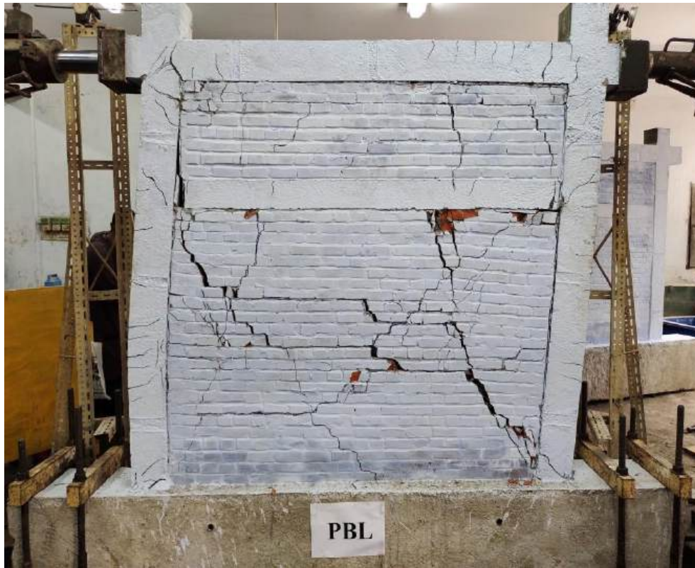
Figure H.13- PBL at complete failure.
