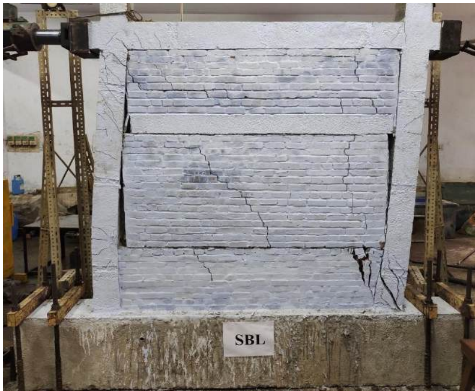
Figure H.12- SBL at complete failure.
