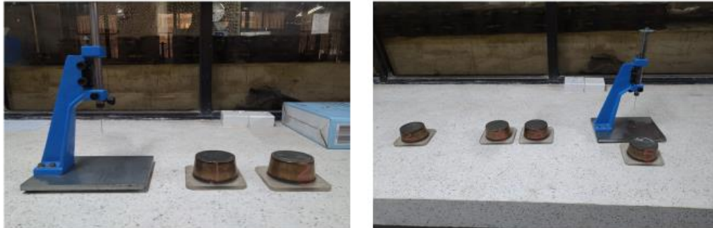
Figure: Determination of initial setting time and final setting time of sample using Vicat's apparatus
