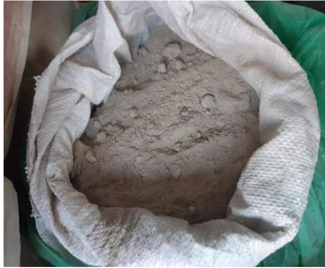
Figure 6.5: LRF slag used as fine aggregate replacement
